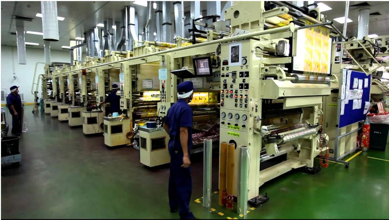
In gravure printing, the image is engraved onto a copper cylinder because, like offset and flexography, it uses a rotary printing press. The vast majority of gravure presses print on reels of paper, rather than sheets of paper. Gravure printing is used for long, high-quality print runs such as magazines, mail-order catalogues, packaging, and printing onto fabric and wallpaper. It is also used for printing postage stamps and decorative plastic laminates, such as kitchen worktops.
